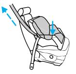
snugness of the child seat to the vehicle. Sometimes, a slight lean towards the buckle will additionally help to remove remaining slack from the belt.
